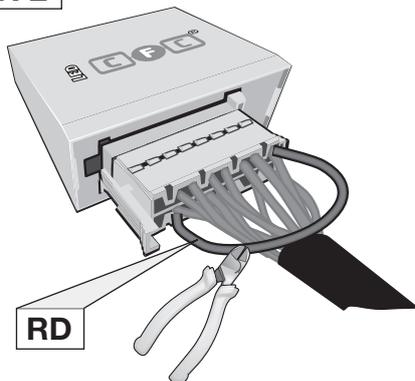
Pin 11 and Pin 2 disconnected
