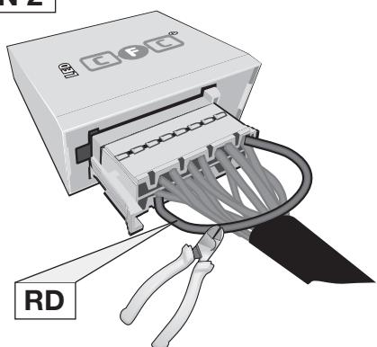
Pin 11 and Pin 2 disconnected
